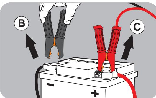
*Disconnect the charger from the mains (A), then remove the black clamp (B) and finally the red clamp (C).*
