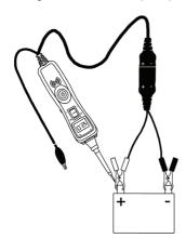
While the Cargo 211097 is in Power Probe Mode, contact the probe tip to a POSITIVE circuit. The red positive sign "+" LED will light and the voltage reading of the circuit will be indicated on the LCD display. If the audio feature is turned on, a high pitched tone will sound.
